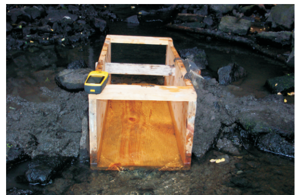
Low stream flows can be determined by measuring water width, depth, and velocity in a wooden flume
