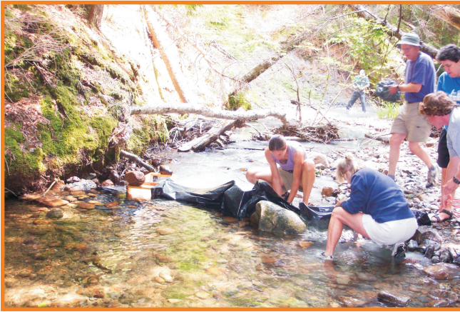
Preparing to measure stream flow using a wooden flume
