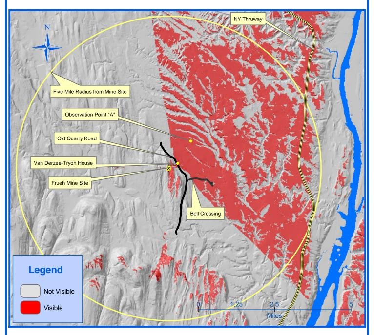
Viewshed Based on Terrain Elevation Only Digital Elevation Model from USGS Projection: NAD 83 Datum: Zone 18 Prepared by HydroQuest June 2003 Paul A. Rubin
